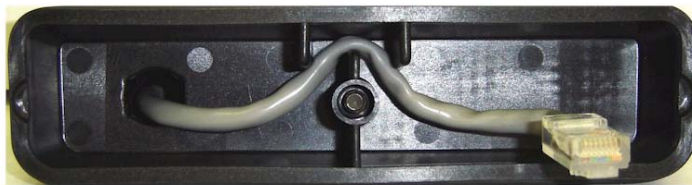
Figure 8: Face Plate Cover Strain Relief
