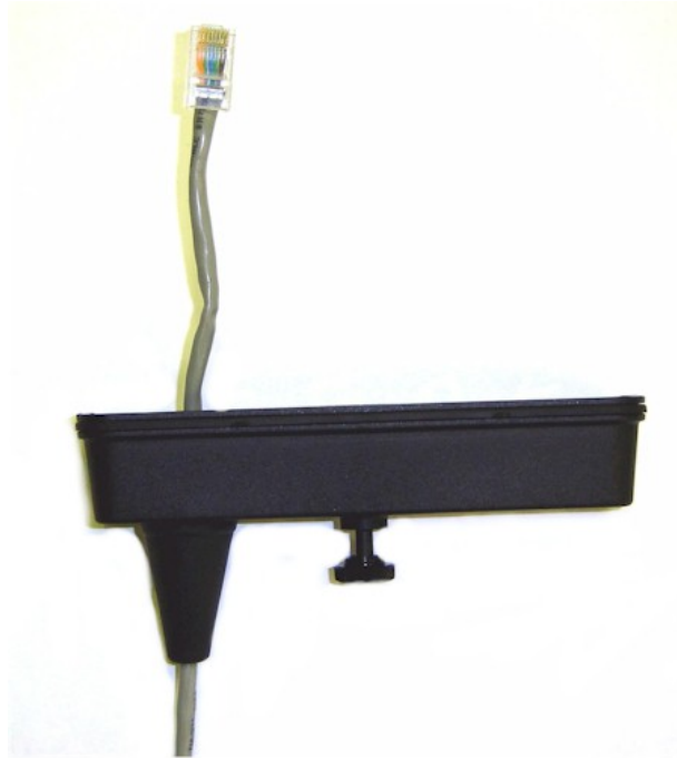
Figure 7: Ethernet Cable Routing
