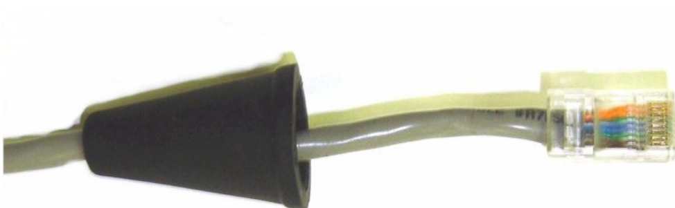
Figure 6: Ethernet Cable Assembly
