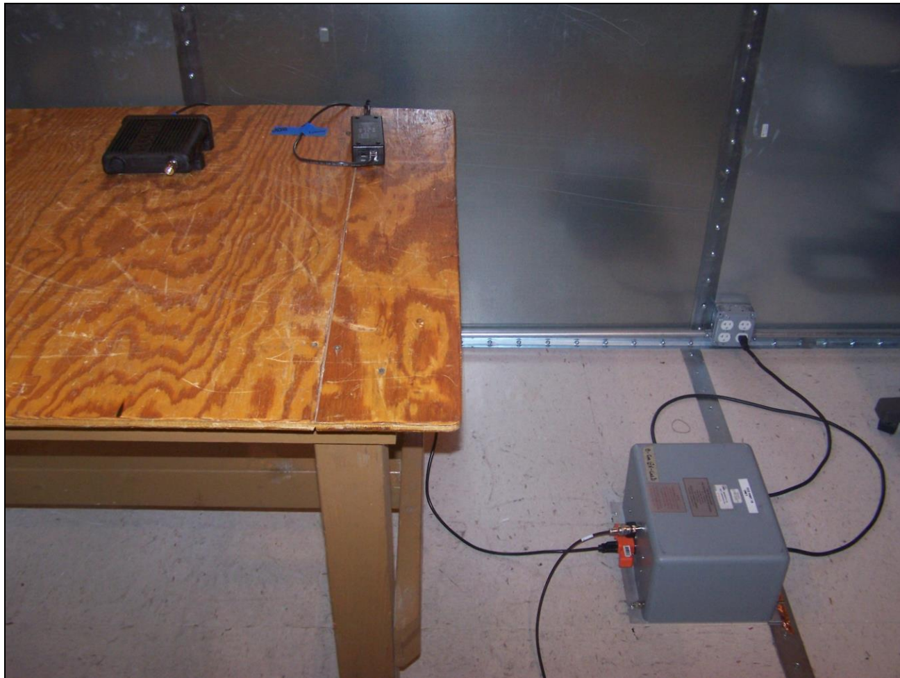
Photograph 1. Conducted Emissions, Test Setup
