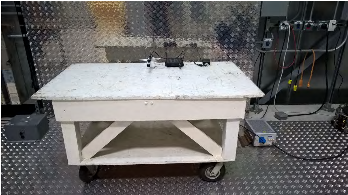
Figure 3.6-3: AC Conducted Emissions Test Setup
