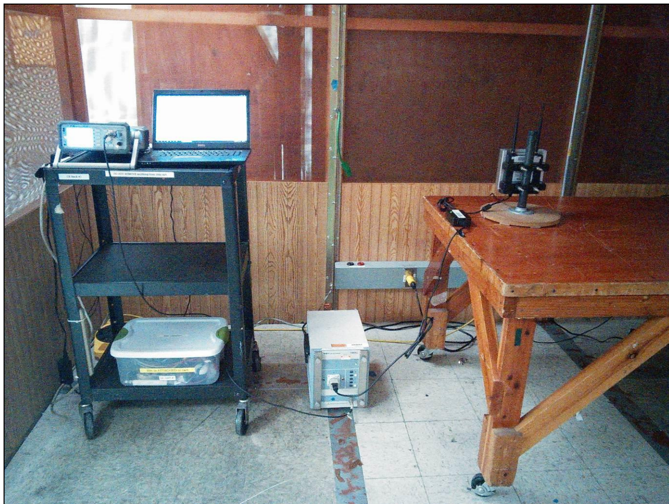
Photograph 4. Conducted Emissions, 15.207(a), Test Setup
