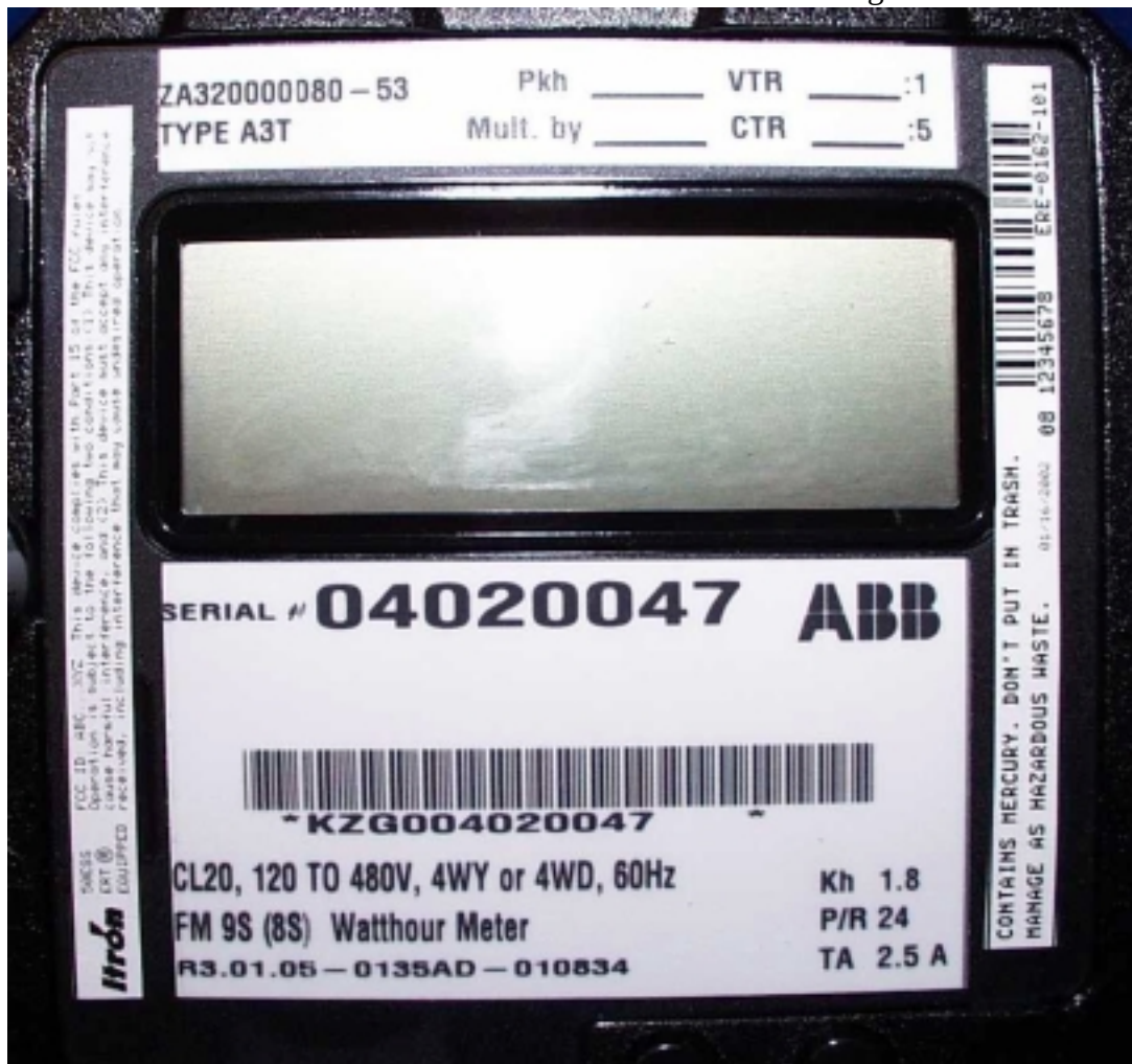
Labels attached to the Internal Meter Housing
