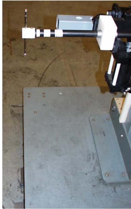
Photo 14 Alignment of the Center of Antenna with the Platform Edge
