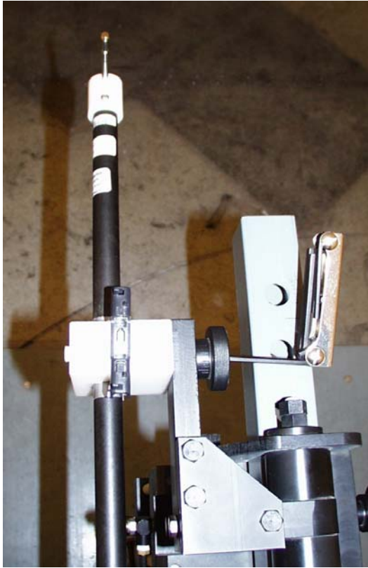
Photo 13 Leveling Using Bubble Level
