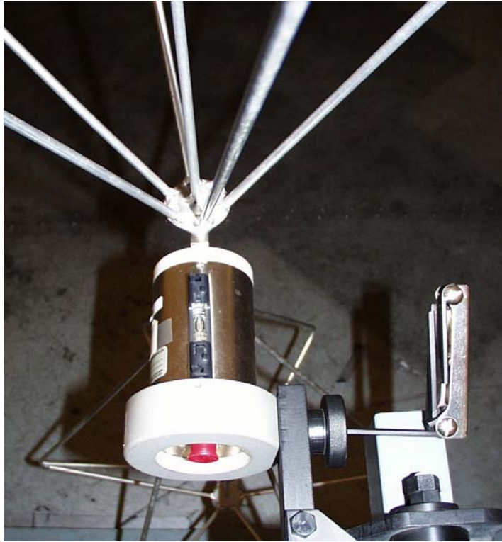
Photo 8 Leveling Using Bubble Level
