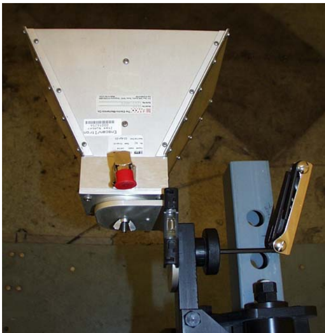
Photo 15 Leveling Using Bubble Level
