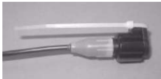
Figure 10: Cable tie on register connector
