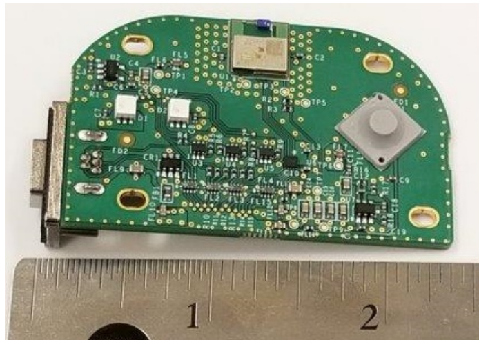
Communications Control Board - Top Side (all devices)
