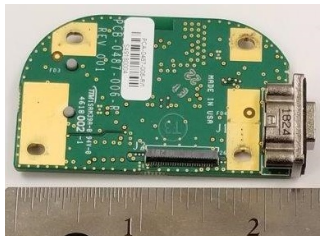
Communications Control Board - Bottom Side (all devices)
