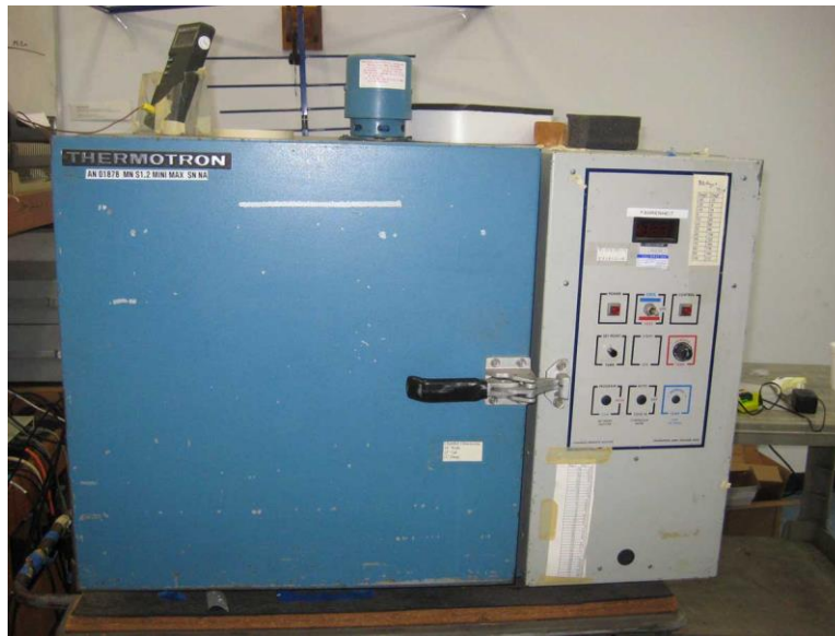
Outside Temperature Chamber
