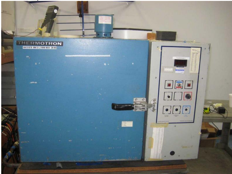
Outside Temperature Chamber
