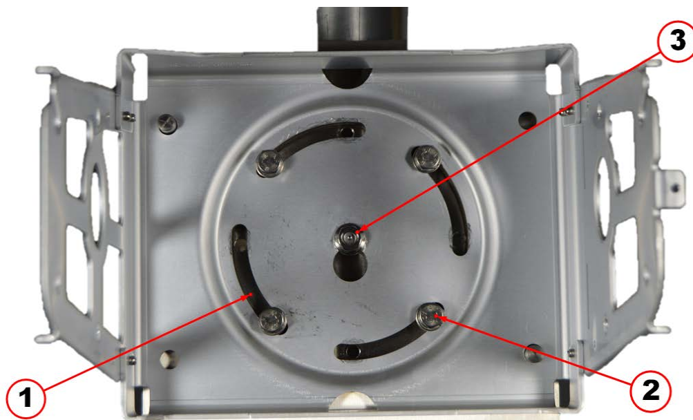
Figure 21 Hex Bolts, Alignment Slots and Self-Locking Hex Bolt Location
