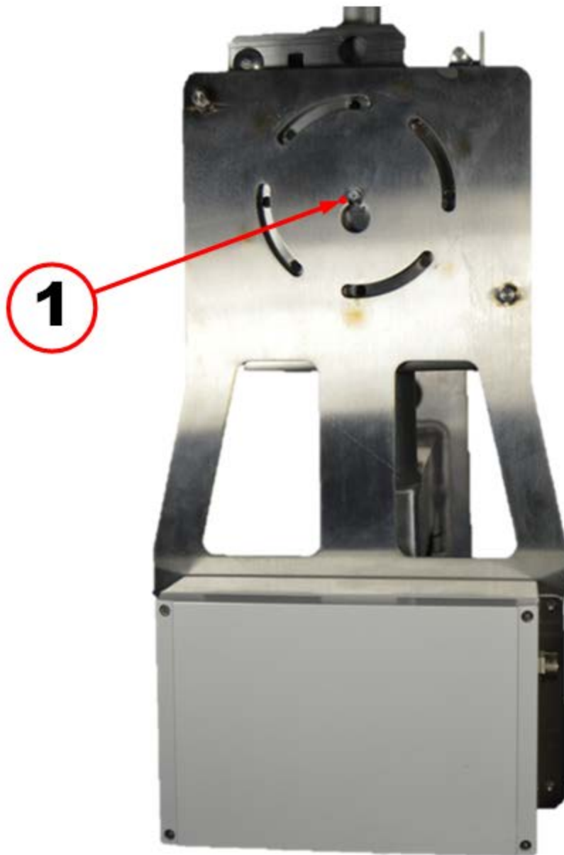
Figure 61 ACT Coupler Unit Mounting Bracket Center Stud with Self-Locking Hex Nut
