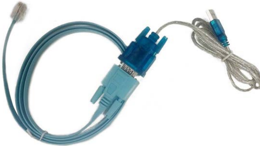
Figure 76 Cisco DB9-RJ45 Serial Cable and USB-to-Serial Adapter Cable
