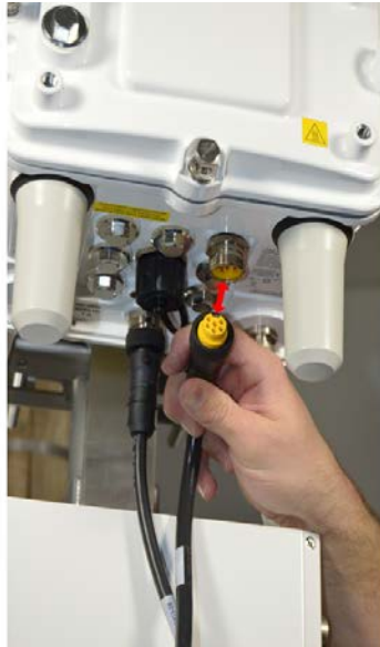
Figure 71 PLC Signal Cable Connection to the CGR Location
