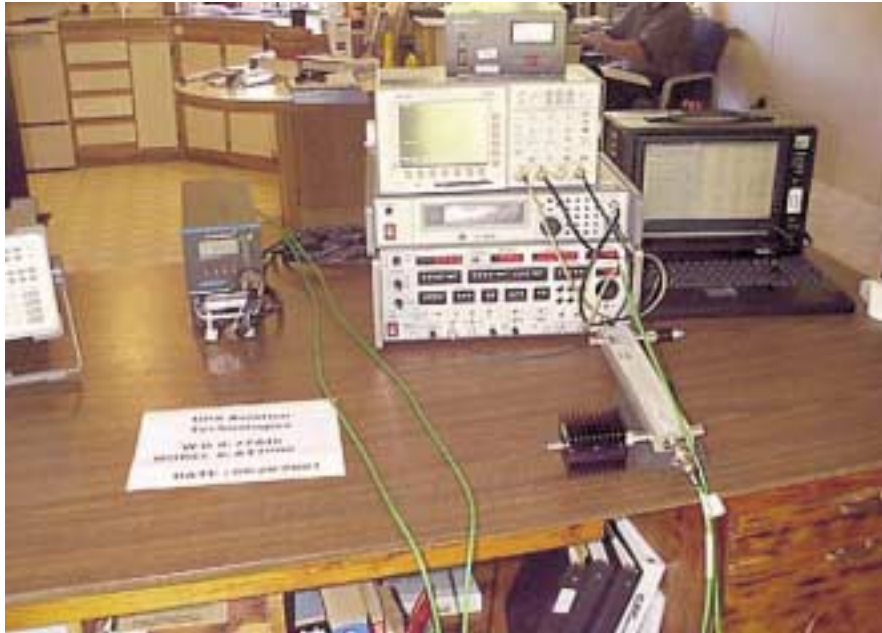
Test Setup of Pulse Width – Front View
