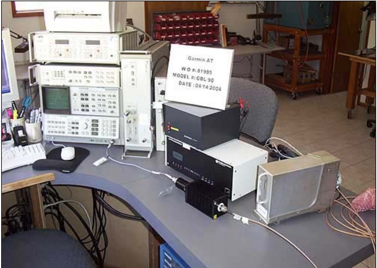
PHOTOGRAPH SHOWING DIRECT CONNECT TEST SETUP
