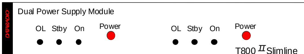
Figure 8 - Dual Power Supply Module front panel
