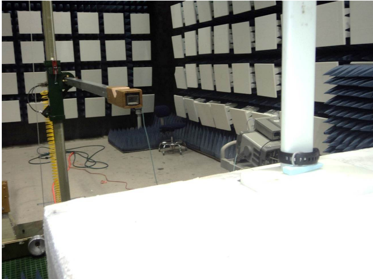
Figure 6: Typical Radiated Emissions – 18 GHz to 24 GHz shown, rear view
