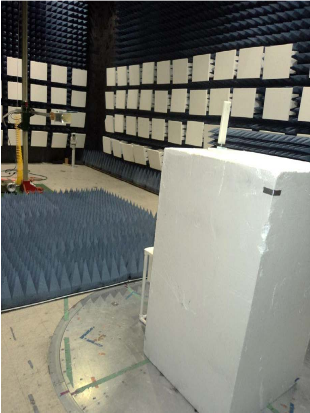
Figure 4: Typical Radiated Emissions – 1 GHz to 18 GHz shown, rear view
