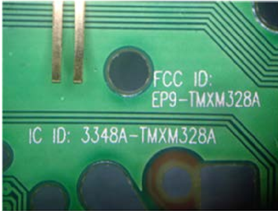
Figure 1: Label Art silk-screened on the watch circuit board.
