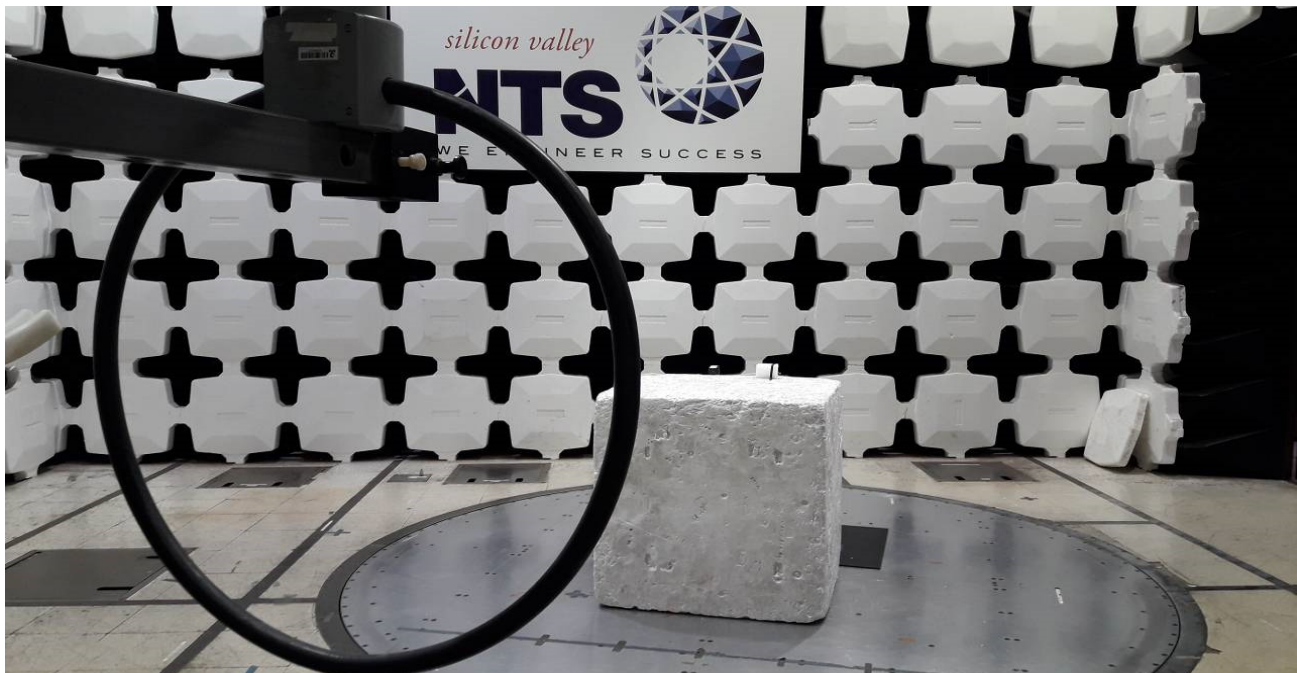
Test Configuration Photograph #1 (Radiated Emissions - Below 30 MHz)
