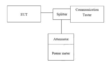
Measurement Setup for testing on Antenna connector.
