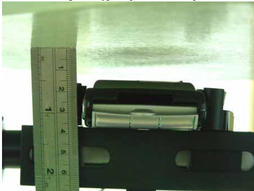
Fig. 9.9 Keypad Down with 1.5cm Gap
