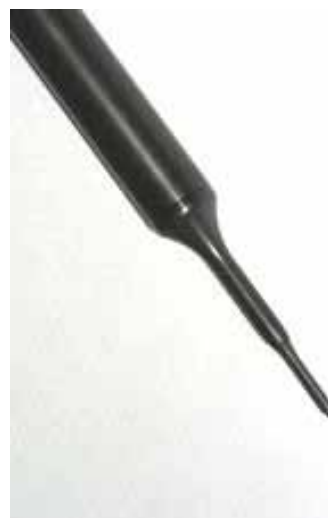
Fig. 5.3 EX3DV4 E-field Probe
