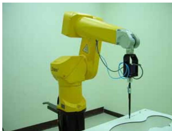
Fig. 5.2 Probe setup on robot
