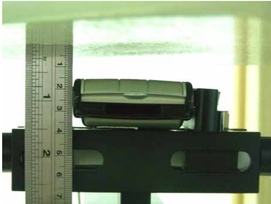
Fig. 9.8 Keypad Up with 1.5cm Gap
