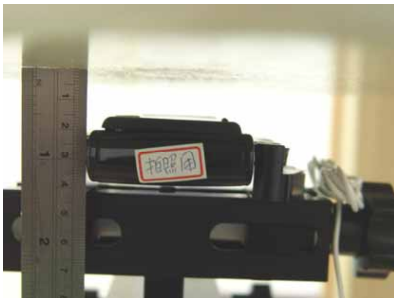
Fig. 9.7 Keypad Down with 1.5cm Gap
