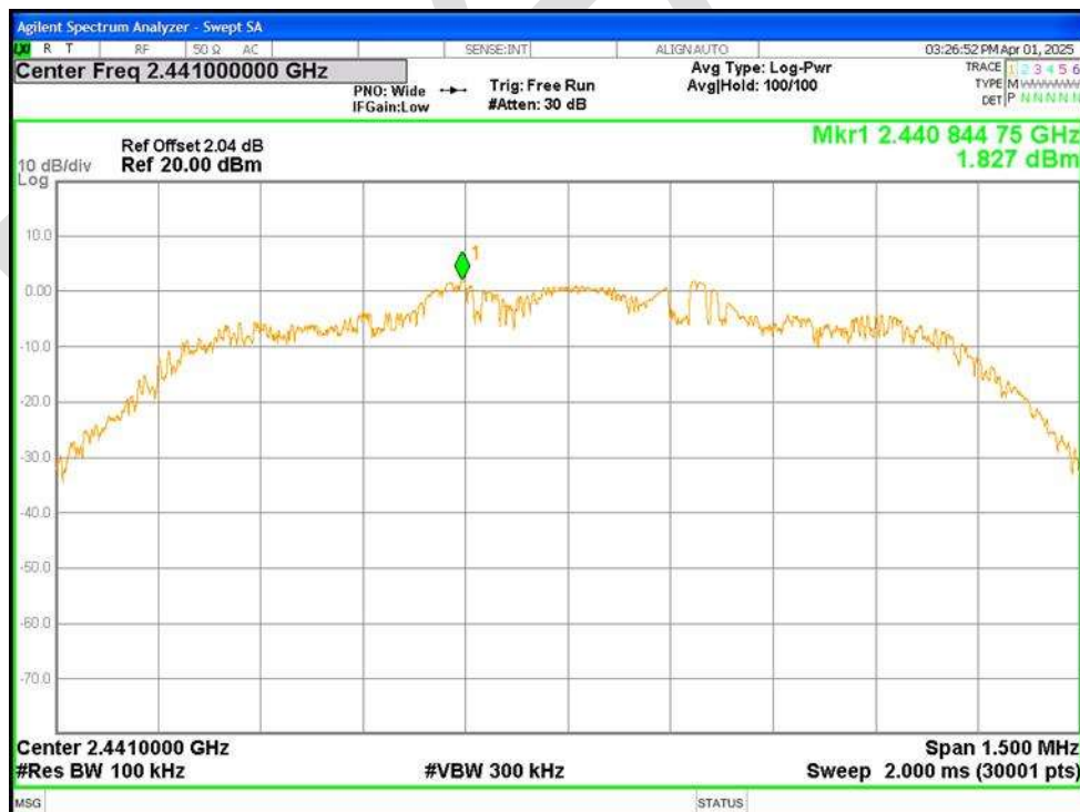
Tx. Spurious NVNT 3-DH1 2441MHz Ant1 Ref
