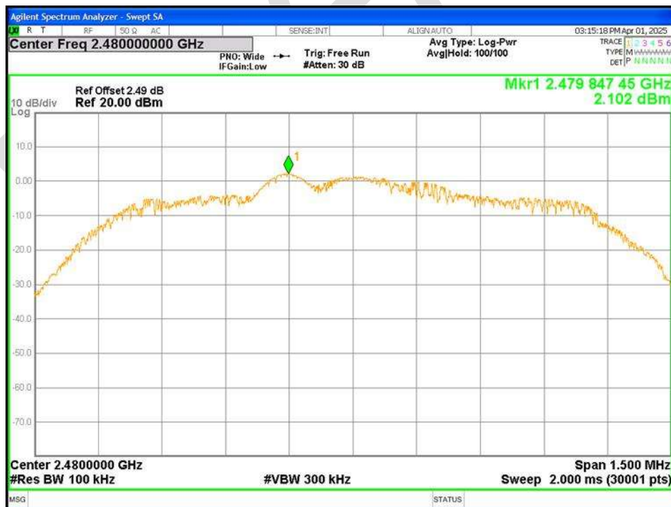
Tx. Spurious NVNT 2-DH1 2480MHz Ant1 Ref
