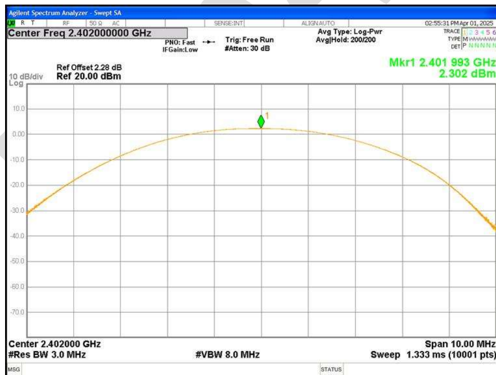
Power NVNT 1-DH1 2402MHz Ant1
