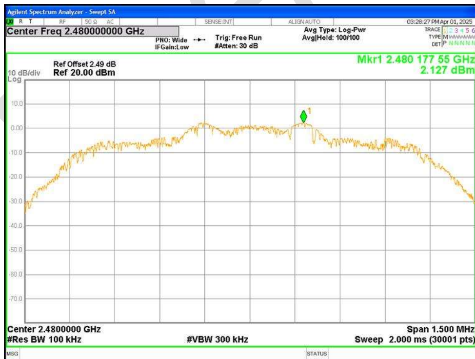
Tx. Spurious NVNT 3-DH1 2480MHz Ant1 Ref
