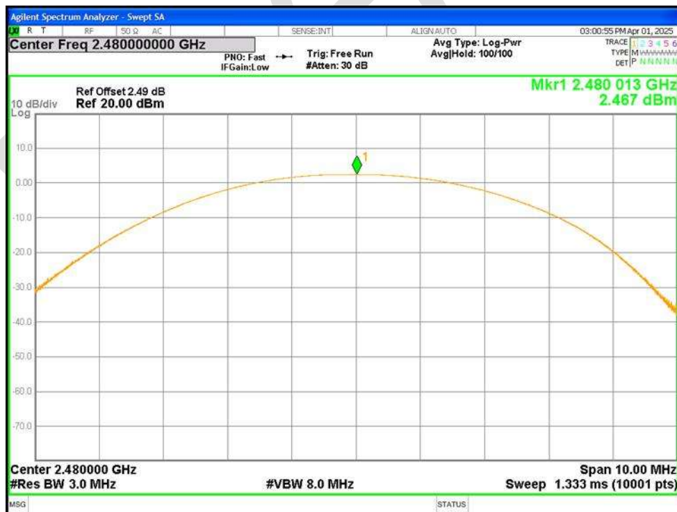
Power NVNT 1-DH1 2480MHz Ant1
