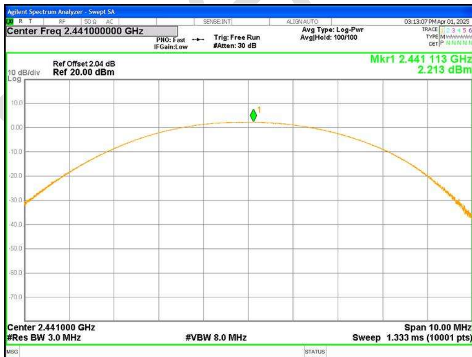
Power NVNT 2-DH1 2441MHz Ant1
