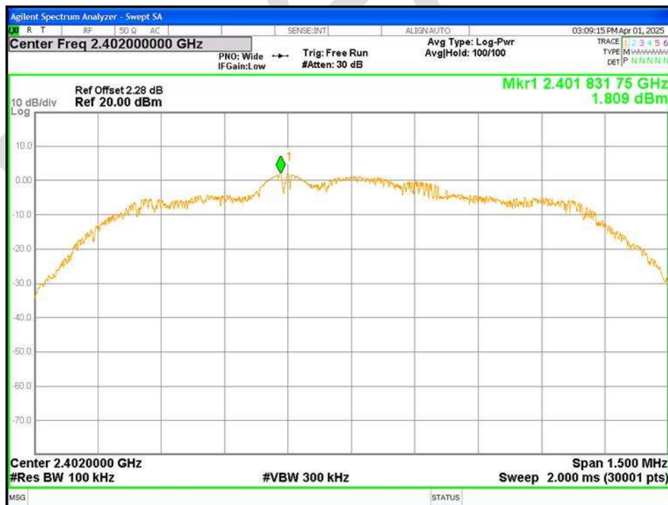
Tx. Spurious NVNT 2-DH1 2402MHz Ant1 Ref
