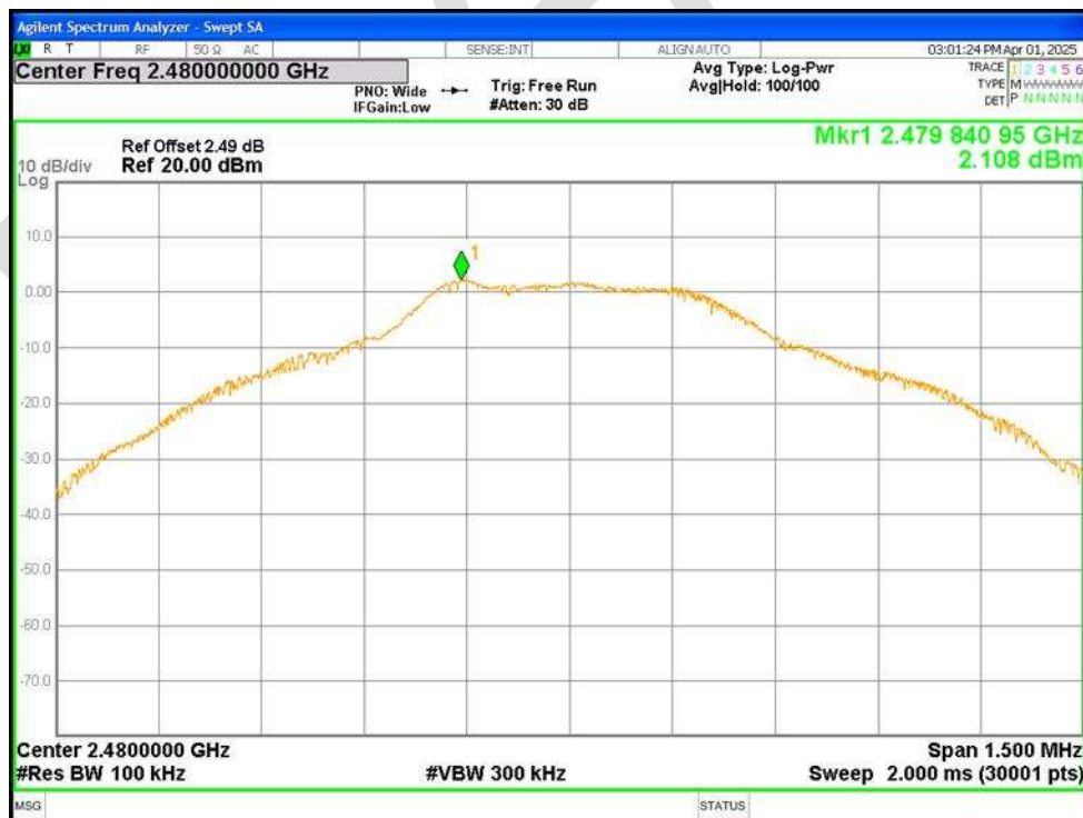
Tx. Spurious NVNT 1-DH1 2480MHz Ant1 Ref
