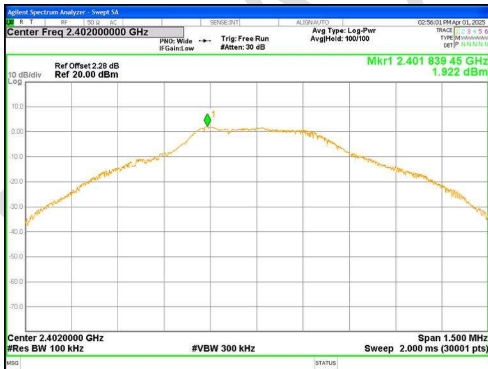
Tx. Spurious NVNT 1-DH1 2402MHz Ant1 Ref
