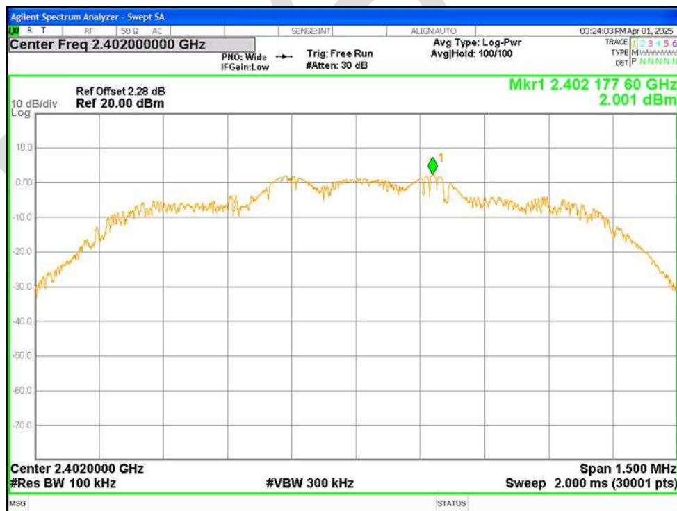
Tx. Spurious NVNT 3-DH1 2402MHz Ant1 Ref
