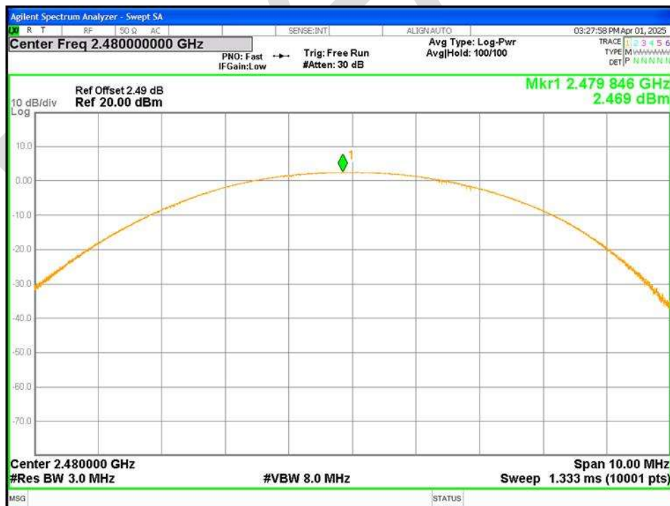
Power NVNT 3-DH1 2480MHz Ant1
