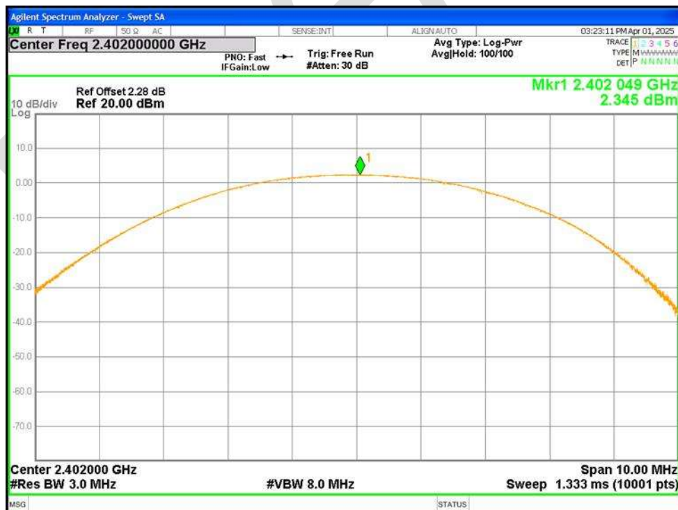
Power NVNT 3-DH1 2402MHz Ant1
