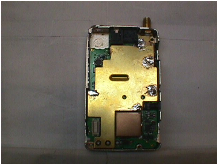
FIGURE 16: Main Board with copper shield
