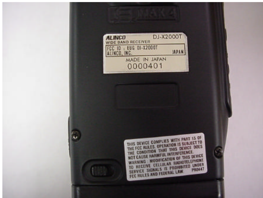
FIGURE 2: LOCATION OF LABELS ON EUT
