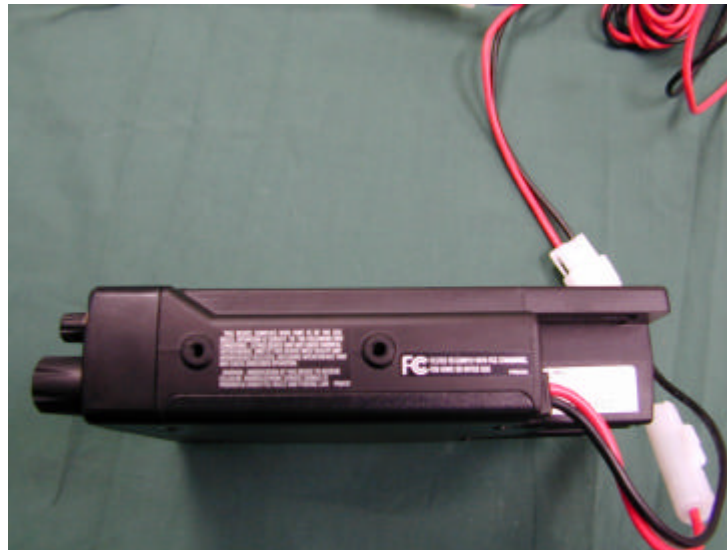
FIGURE 2: LOCATION OF LABELS ON EUT
