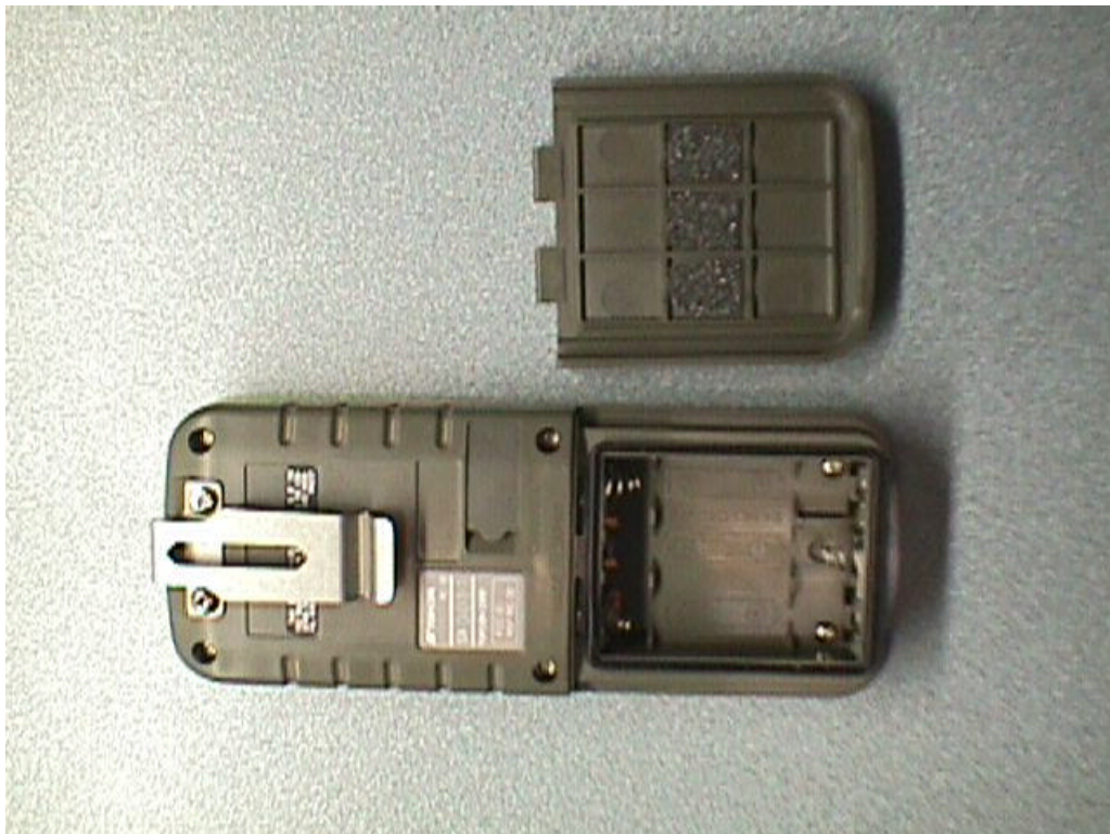
REAR VIEW OF BATTERY COMPARTMENT
