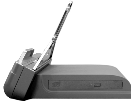
Figure 3.6.2 The side view of the docking station
