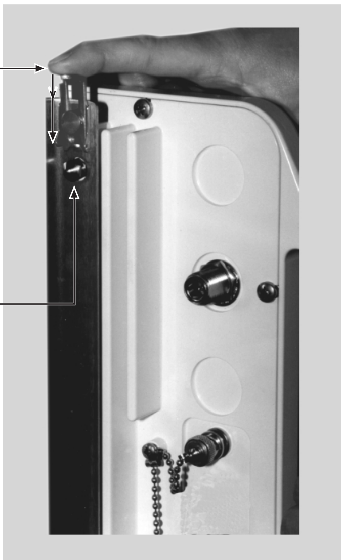
Figure 3.3b - Locking the Mounting Hardware
