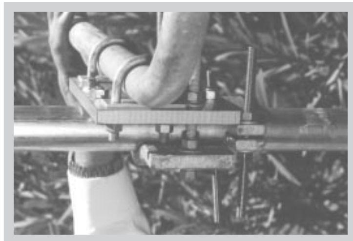
Figure B.16 - Azimuth Adjustment Clamp Assembly
