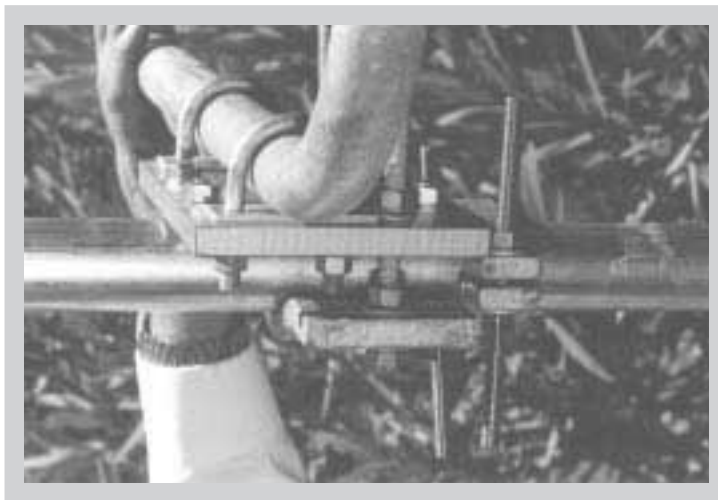
Figure 4.21 - Azimuth Adjustment Clamp Assembly
