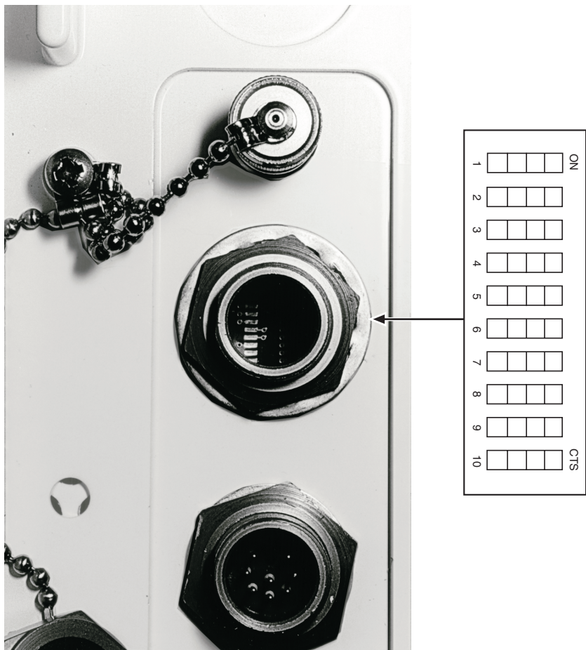
Figure 3.8 - DIP Switch Access and Configuration Information
