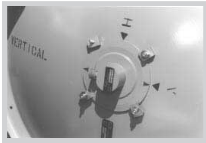
Figure 4.19 - Feed Horn Installation for Vertical Polarized Operation
