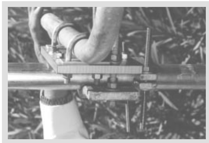
Figure B.16 - Azimuth Adjustment Clamp Assembly
