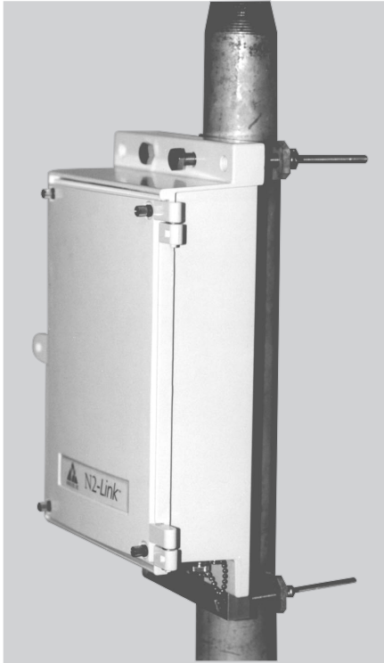
Figure 3.3a - V-Clamps and Hardware
