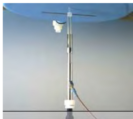
Photograph of the dipole Antenna
