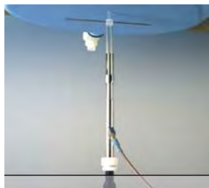
Photograph of the dipole Antenna
