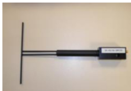
Figure 1 – Satimo COMOSAR Validation Dipole
