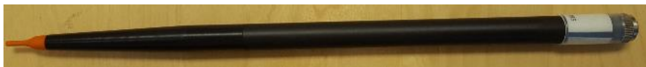
Figure 1 – MVG COMOSAR Dosimetric E field Dipole
