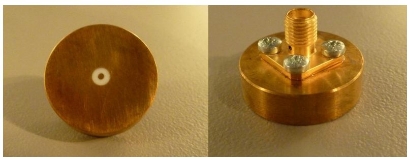
Figure 1 – MVG LIMESAR Dielectric Probe
