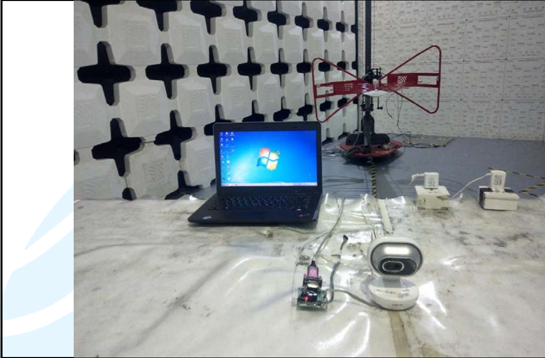
Radiated emission Test Setup (30 MHz~1 GHz)
