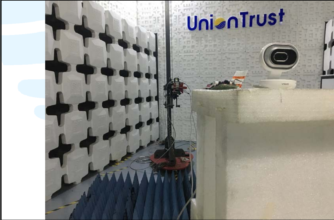
Radiated emission Test Setup (Above 1 GHz)
