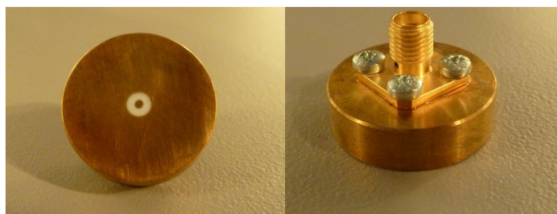
Figure 1 – MVG LIMESAR Dielectric Probe
