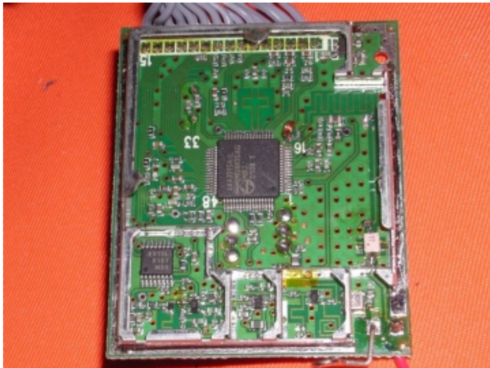
Handset Oscillator PCB comp side
