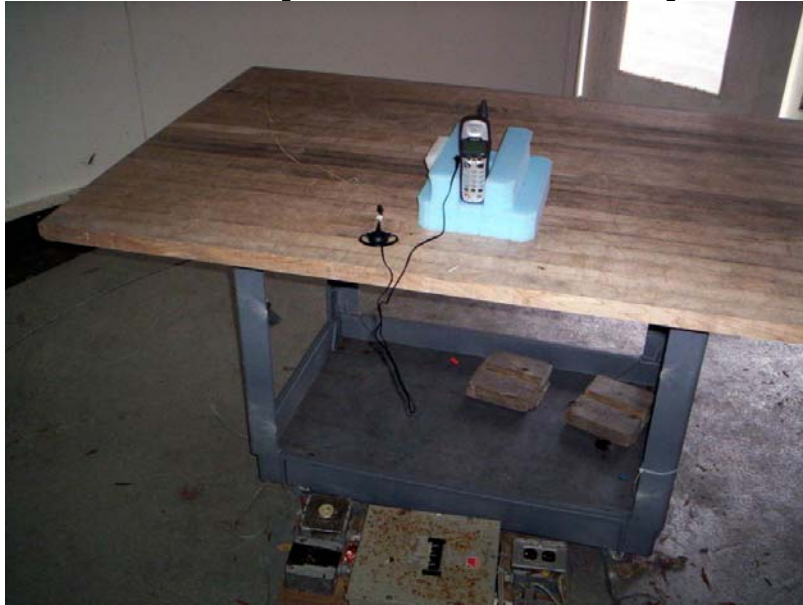
Radiated Spurious Emissions Test Setup
