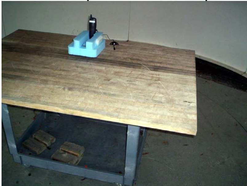
Radiated Spurious Emissions Test Setup
