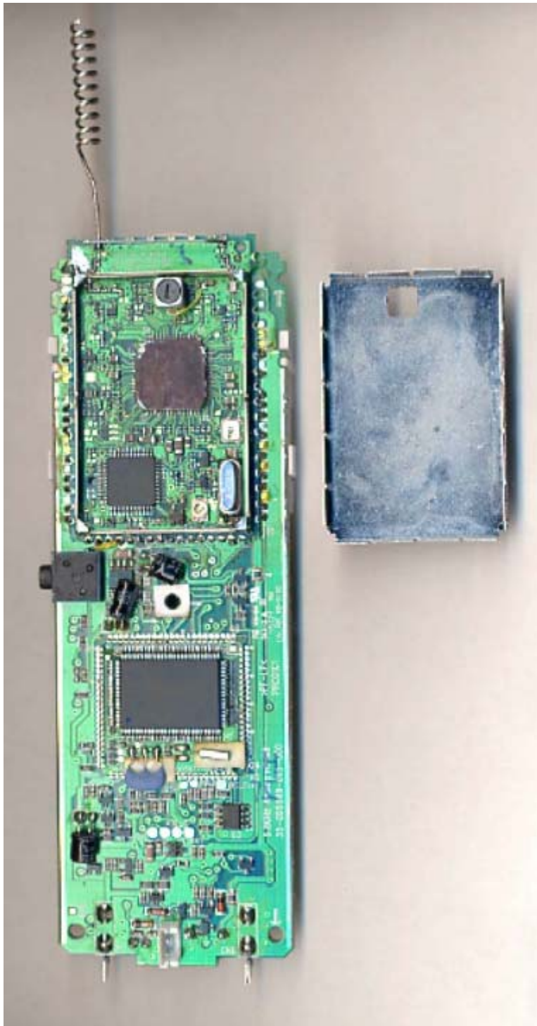
EUT – Component Shielding Off View
