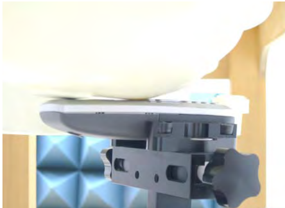
Figure 13. Right Head SAR Test Setup (Cheek)
