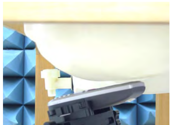
Figure 16. Left Head SAR Test Setup (Tilted)
