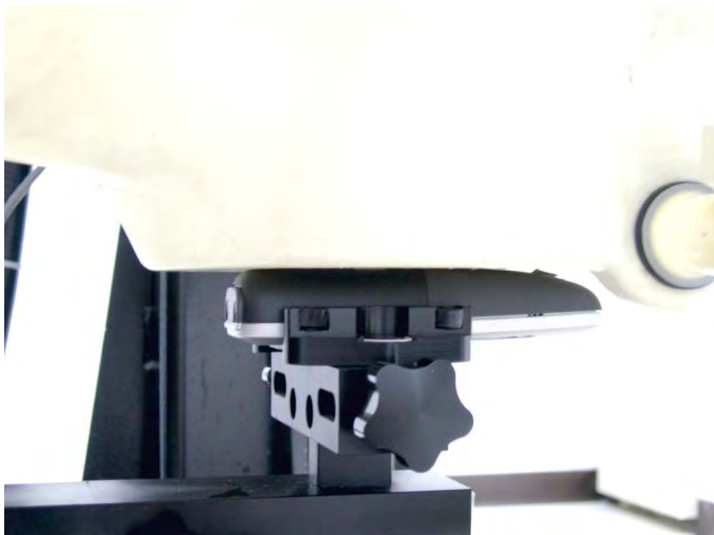
Figure 25. Body SAR Test Setup (Flat Section)
