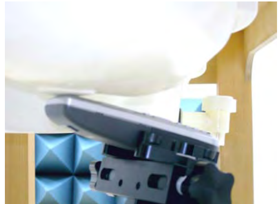
Figure 14. Right Head SAR Test Setup (Tilted)
