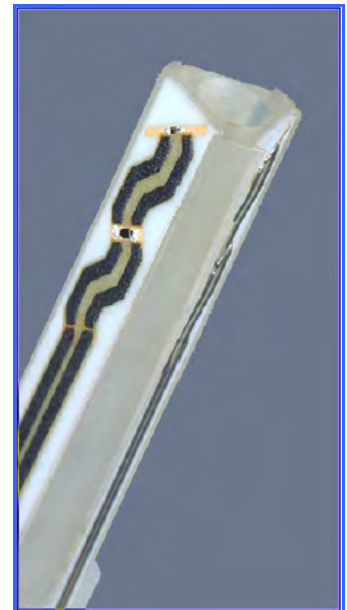
Figure 6. EX3DV3 E-field Probe
