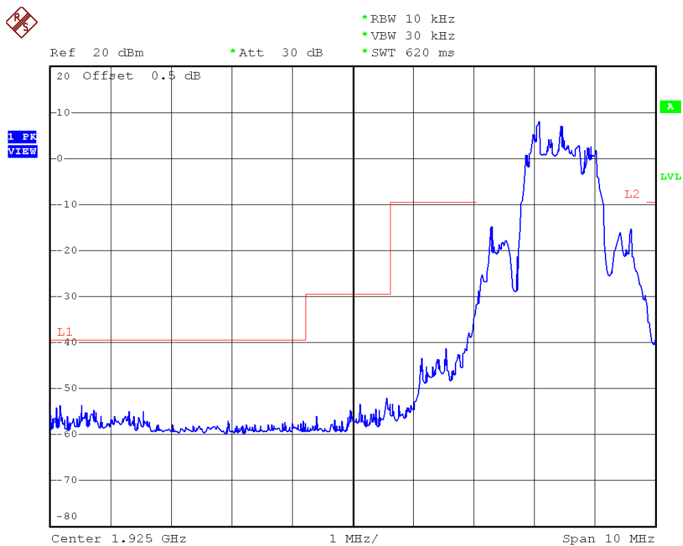
Plot 4B. Highest Channel Unwanted Emission Inside the Sub-Band (Traffic Carrier)
