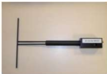
Figure 1 – Satimo COMOSAR Validation Dipole
