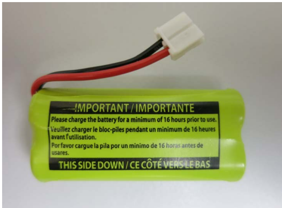
Figure 4 – 2.4V 500mAh Ni-MH Corun rechargeable battery back view
