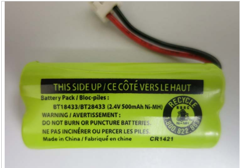
Figure 3 – 2.4V 500mAh Ni-MH Corun rechargeable battery front view
