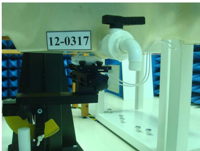
Figure 5. Muscle SAR Test Setup (Flat Section)
