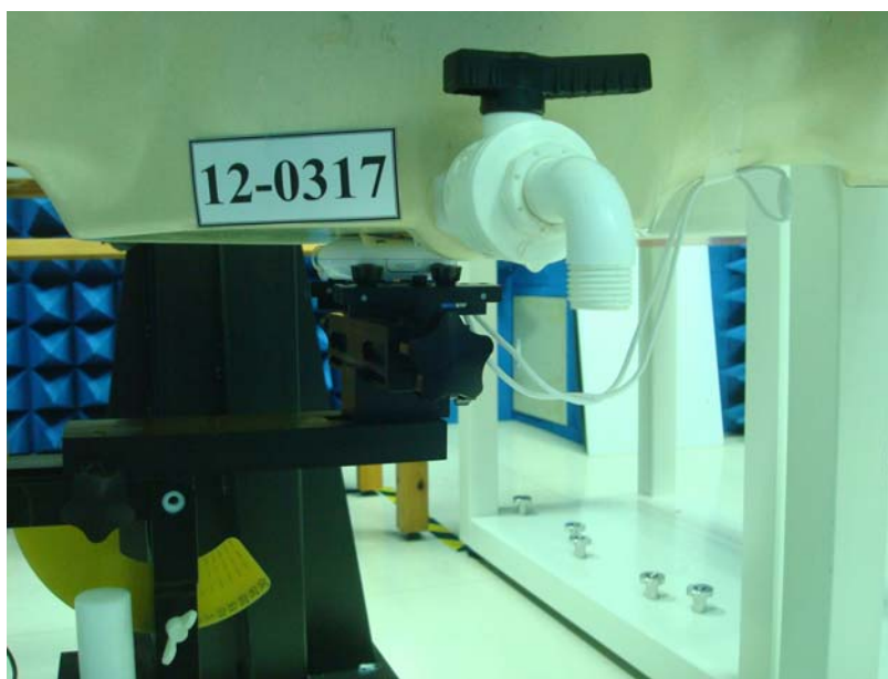
Figure 3. Muscle SAR Test Setup (Flat Section)
