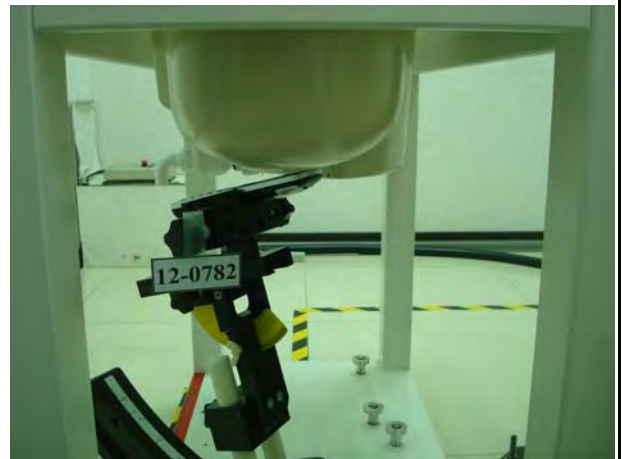
Figure 5. Left Head SAR Test Setup (Tilted)
