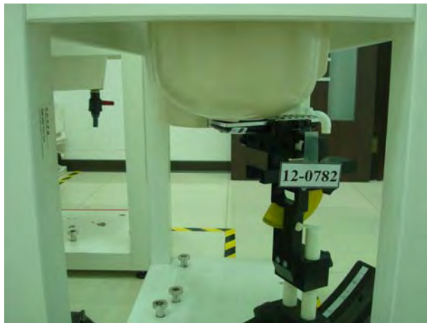
Figure 2. Right Head SAR Test Setup (Cheek)
