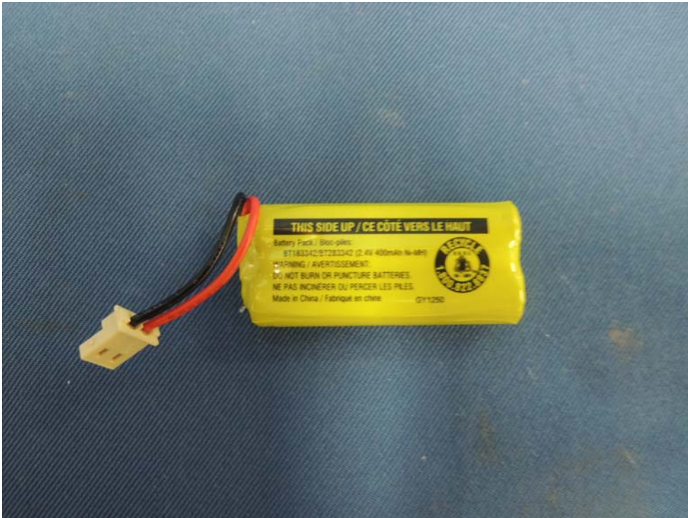
Figure 11 – 2.4V 400mAh Ni-MH Coslight rechargeable battery front view
