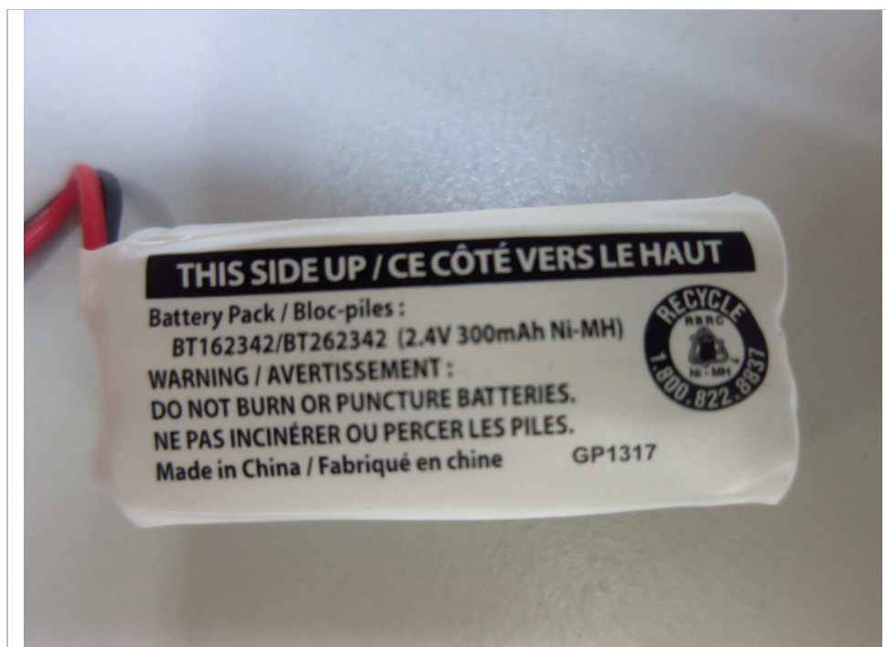
Figure 5 – 2.4V 300mAh Ni-MH GPI rechargeable battery front view
