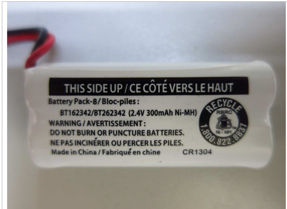
Figure 3 – 2.4V 300mAh Ni-MH Corun rechargeable battery front view
