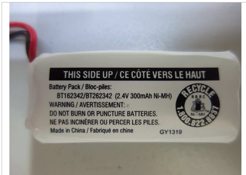
Figure 11 – 2.4V 300mAh Ni-MH Coslight rechargeable battery front view
