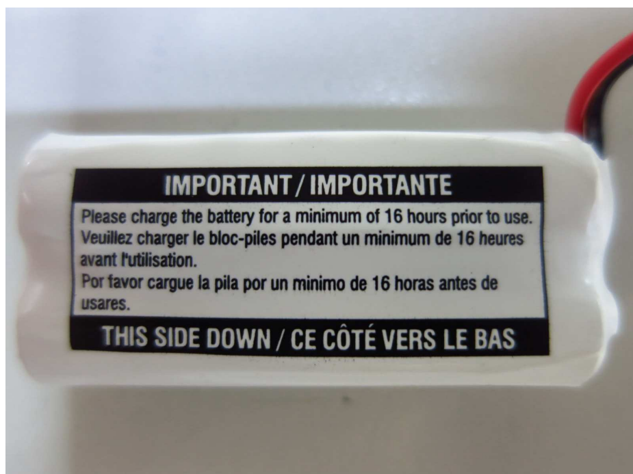
Figure 12 – 2.4V 300mAh Ni-MH Coslight rechargeable battery back view
