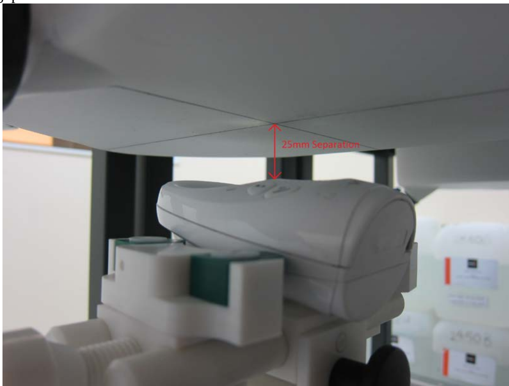
Figure 1 – Front surface with 25mm Separation
