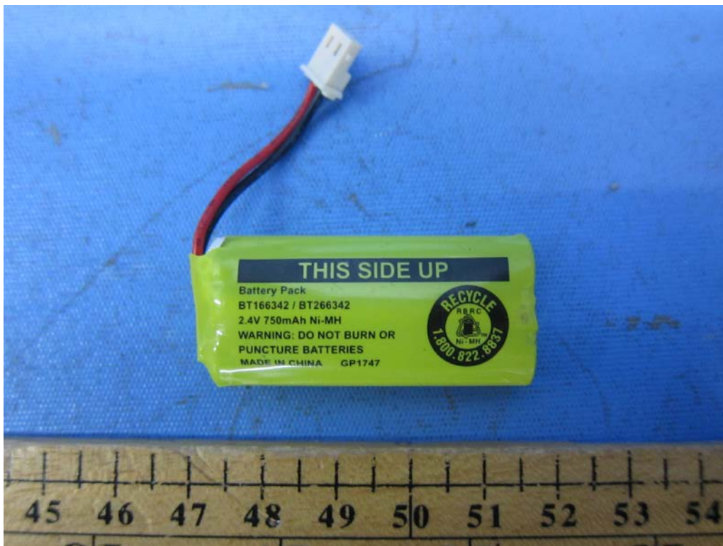
Figure 4 - 2.4V 750mAh GPI Ni-MH rechargeable battery
