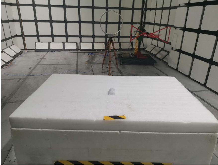
Radiated Emissions View (Below 30MHz)
